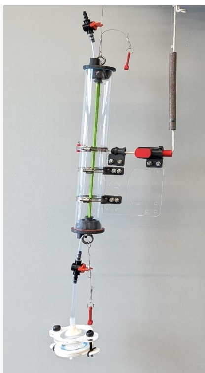
Figure 4.3: A picture of a Van Dorn sampler with modified filtration system
