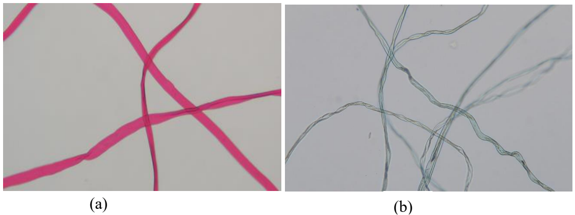
Figure 2.4: Images of (a) Delustrated acrylic fibre (b) Featureless polyester fibre (x400 magnification).
