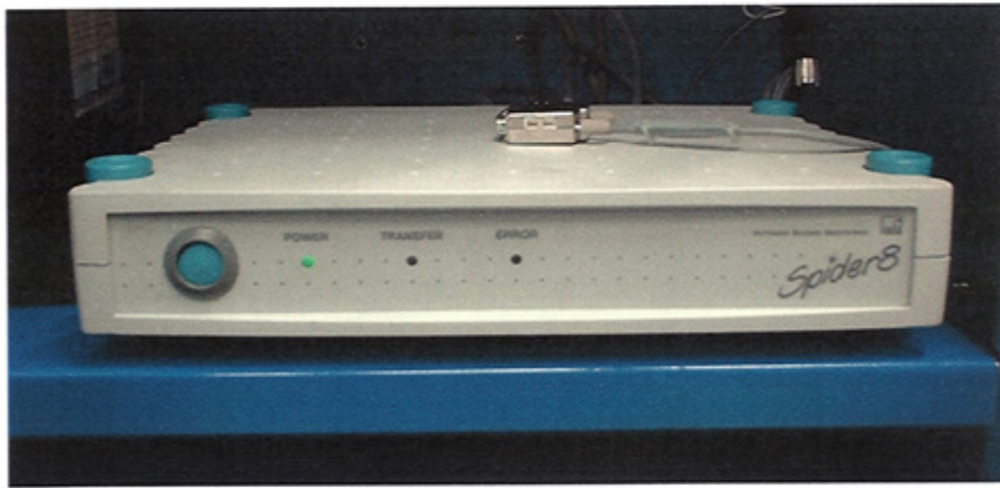
Figure 16 Data logging device, HBM Spider 8.
