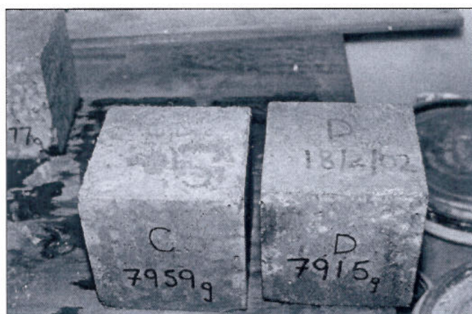
Plate 4 Cubes C and D during freeze/thaw tests at 70 freeze/thaw cycles
