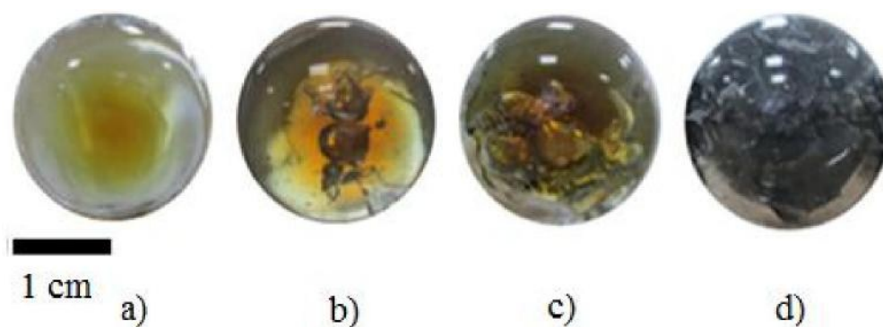
Figure 4. Digital camera captured images of bottoms of the microwaved glass tubes showing: a) neat Epoxy 1; b) Epoxy 2; c) Epoxy 3; and d) Epoxy 4.
