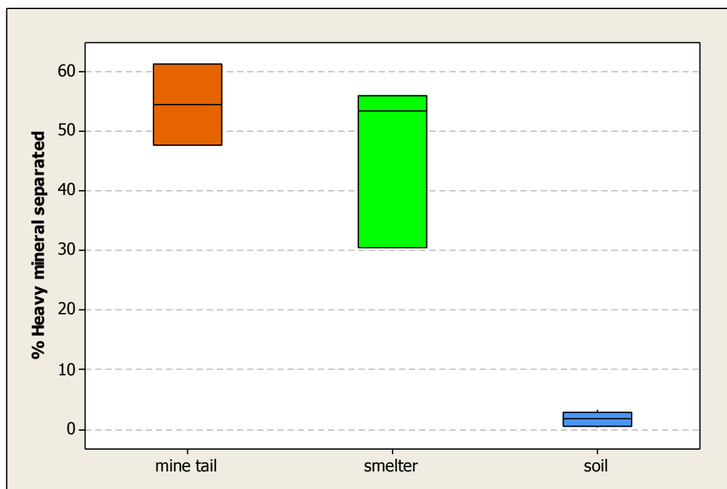
Figure 3.10: Boxplot of % heavy mineral separated from matrices
