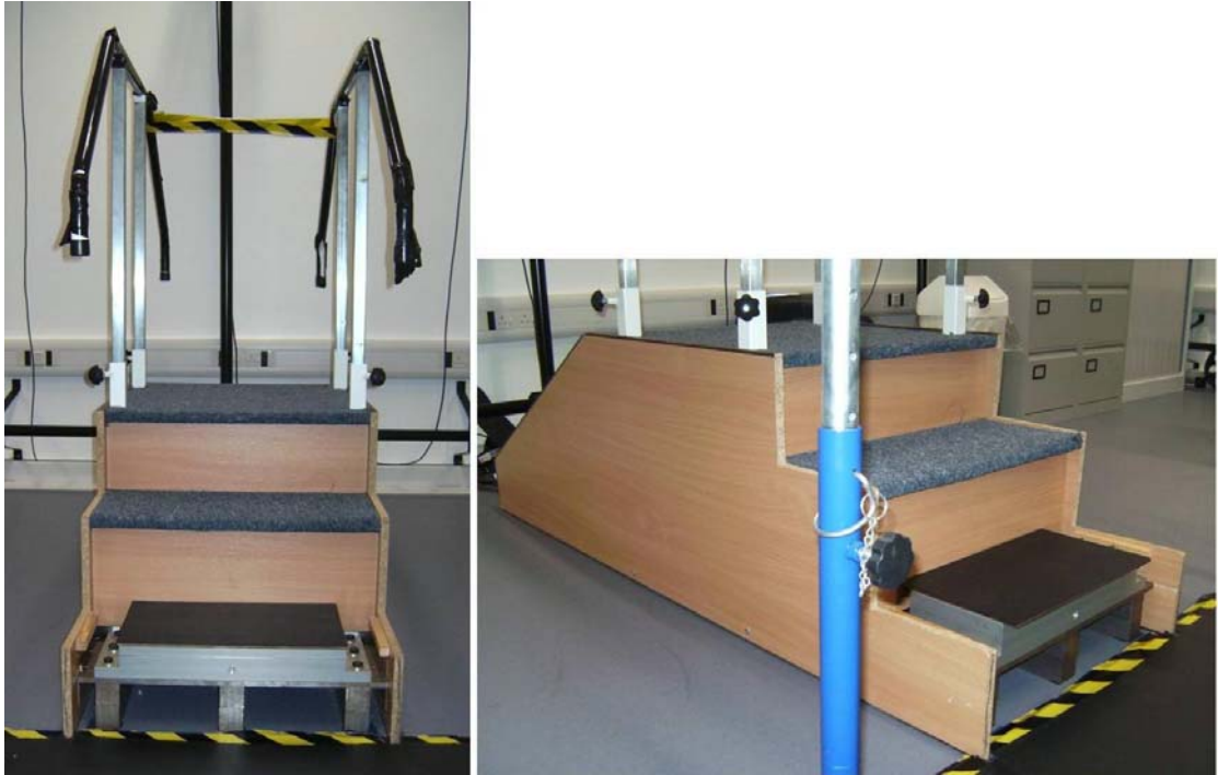
Figure 3.4 The instrumented staircase showing the MC818 force plate.
