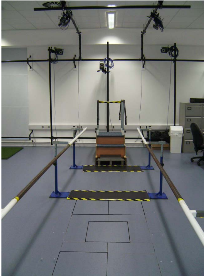
Figure 3.8 The handrails in position in the laboratory showing the free standing handrails and the extension bars covering the force plate area.
