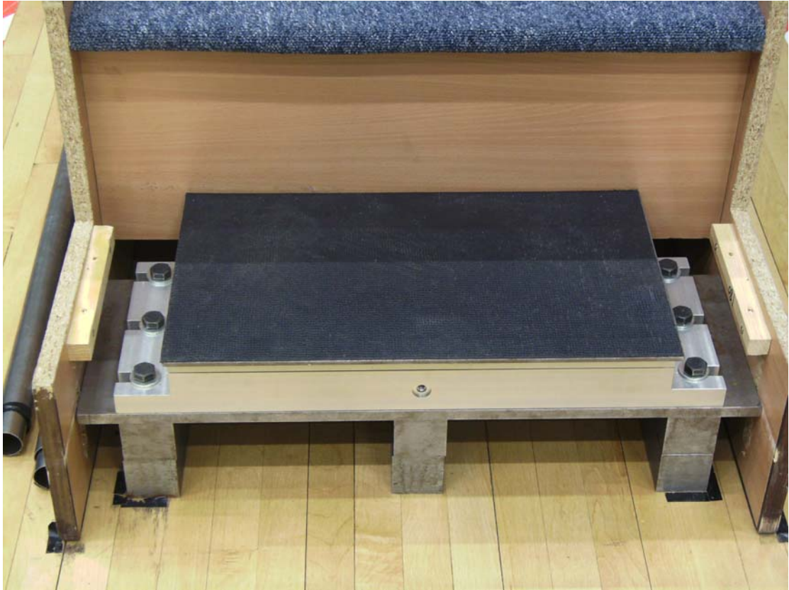
Figure 3.6 Step pedestal shown in position in the staircase.
