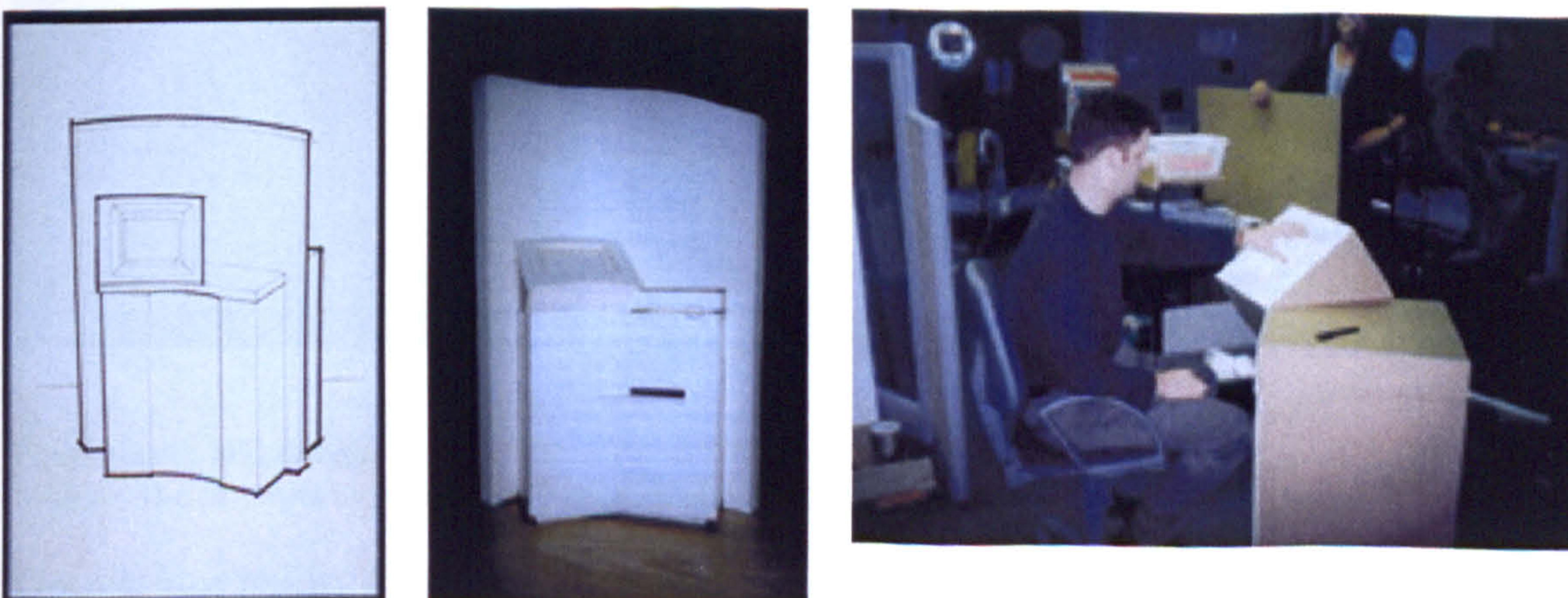
Fig. 58. Left: development drawing of asymmetric concept. Middle: Scale model. Right: Full size test rig.
