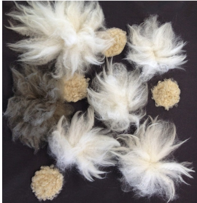
Figure 4. Sheepskin shapes bonded to adhesive prior to trimming.
