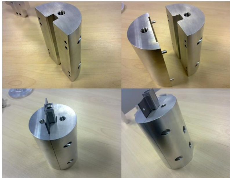
Figure A- 3 Welding fixtures to assist welding fill tube to the SLM HP
