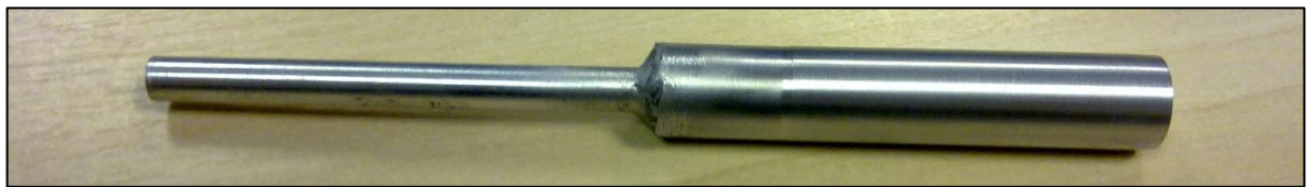
Figure 5- 3 Fill tube welded to the SLM HP
