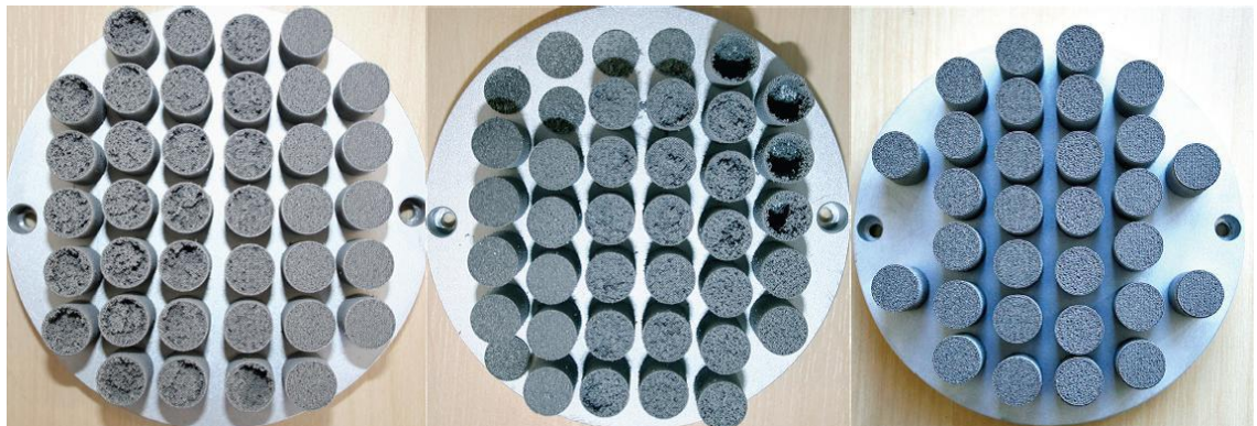
Figure 4-19 Porous samples made for permeability measurements. Different tries improved the quality as shown above from first build at the left to the 3rd build at the right
