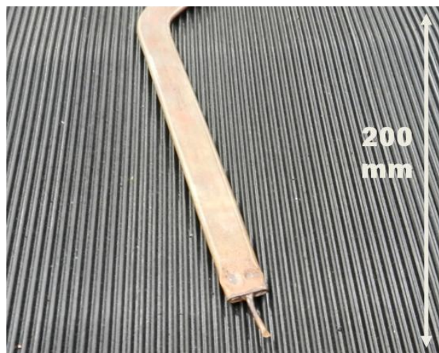
Figure 3- 9 A flattened heat pipe with the fill tube at the end. Fill tube is used to inject the working fluid into the pipe
