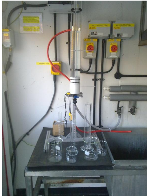
Figure 4- 26 Permeability measurement test rig
