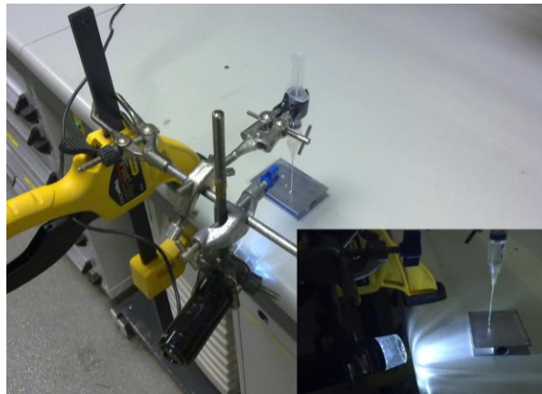
Figure A- 9 Contact measurement test set up
