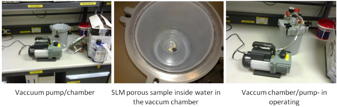
Figure 4- 28 Porosity measurement process
