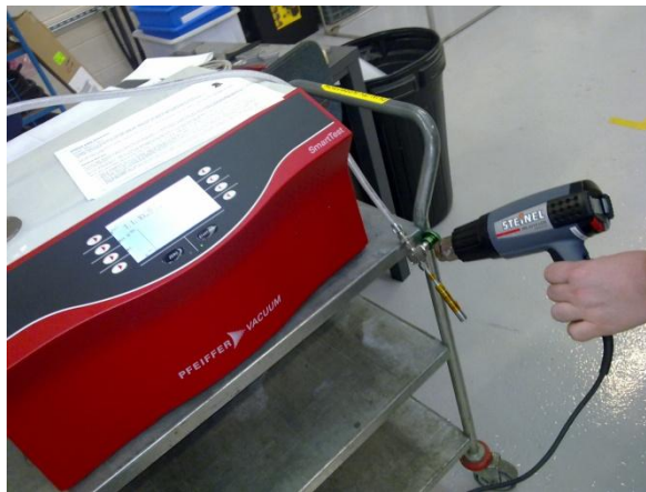
Figure 5- 5 Heat pipe sample is being tested on helium leak testing machine while is being heated by hot air gun to facilitate the extraction of any possible air trapped in the pores
