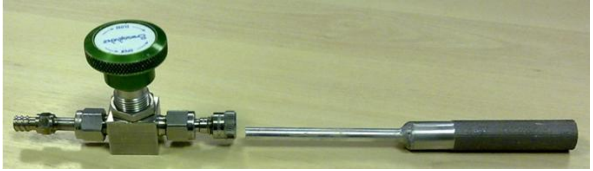
Figure 5- 4 SLM HP, fill tube and valve assembly
