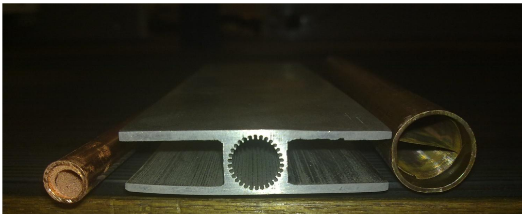
Figure 3- 7 Three major wick types. Left is a copper heat pipe with sintered wick, an aluminium heat pipe with grooved wick is shown in the middle and a copper screen mesh pipe at the right
