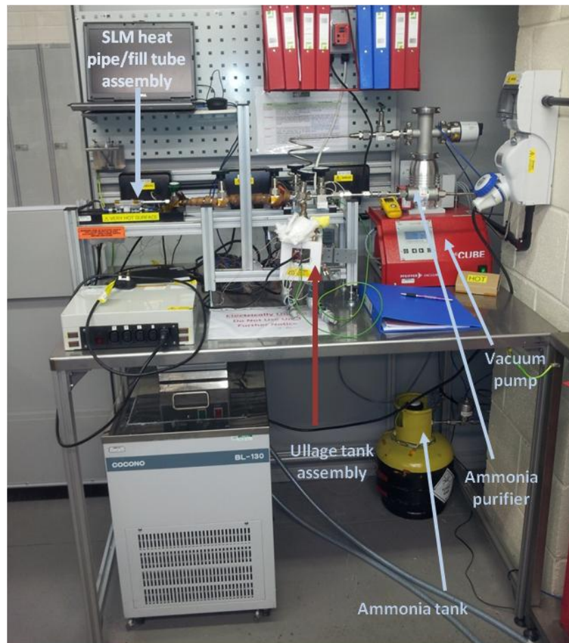
Figure A- 15 Completed ammonia filling rig to fill ammonia into SLM HPs
