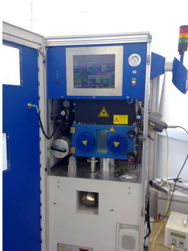
Figure 4-3 SLM 100 machine used for producing the SLM HP prototypes
