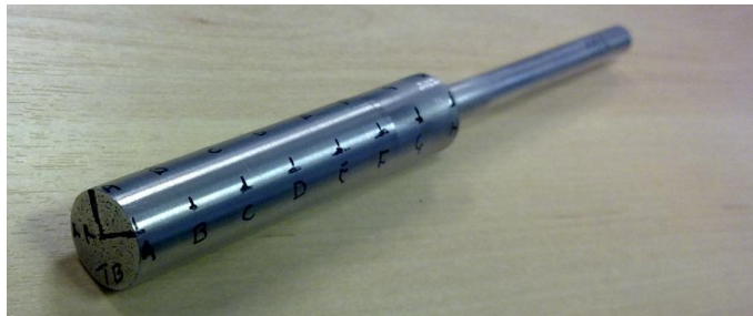
Figure A- 17 Dimension measuring points on the sample before and after proof pressure test
