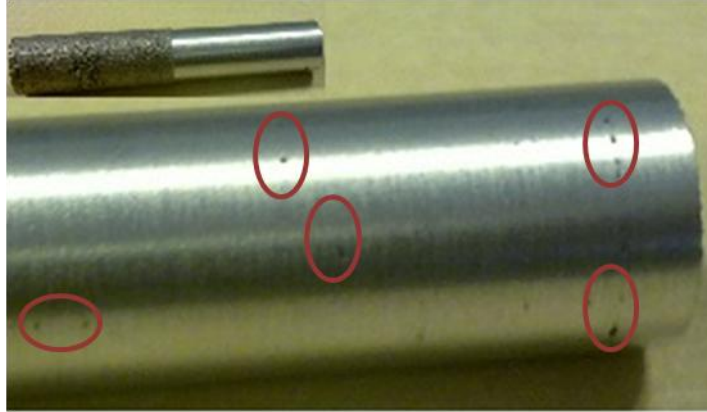
Figure 4- 39 Remaining pores in the initial SLM HP prototypes
