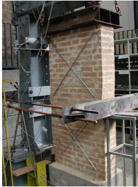
Fig. 3 Typical layout of a shear-compression test.
