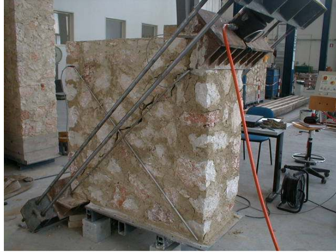
Fig. 1 Typical layout of a diagonal compression test.
