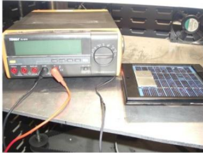
Fig. 4.18: Solid patch element placed upon a poly-Si solar panel for solar measurements in a solar chamber.
