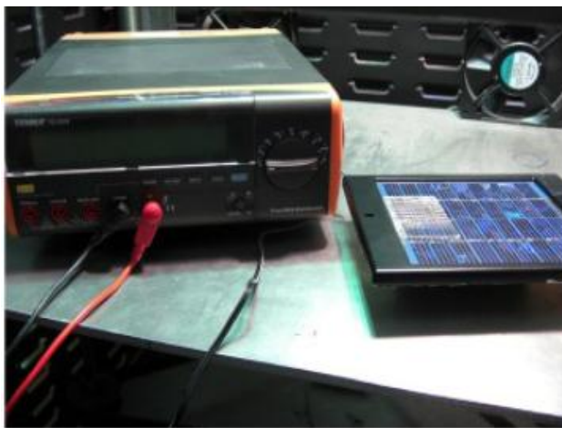
Fig. 4.17: Proposed transparent meshed patch element placed upon a poly-Si solar panel for solar measurements in a solar chamber.
