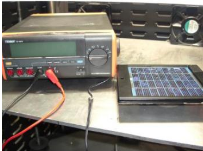
Fig. 4.19: A poly-Si solar panel without any elements placed upon for solar measurements in a solar chamber.
