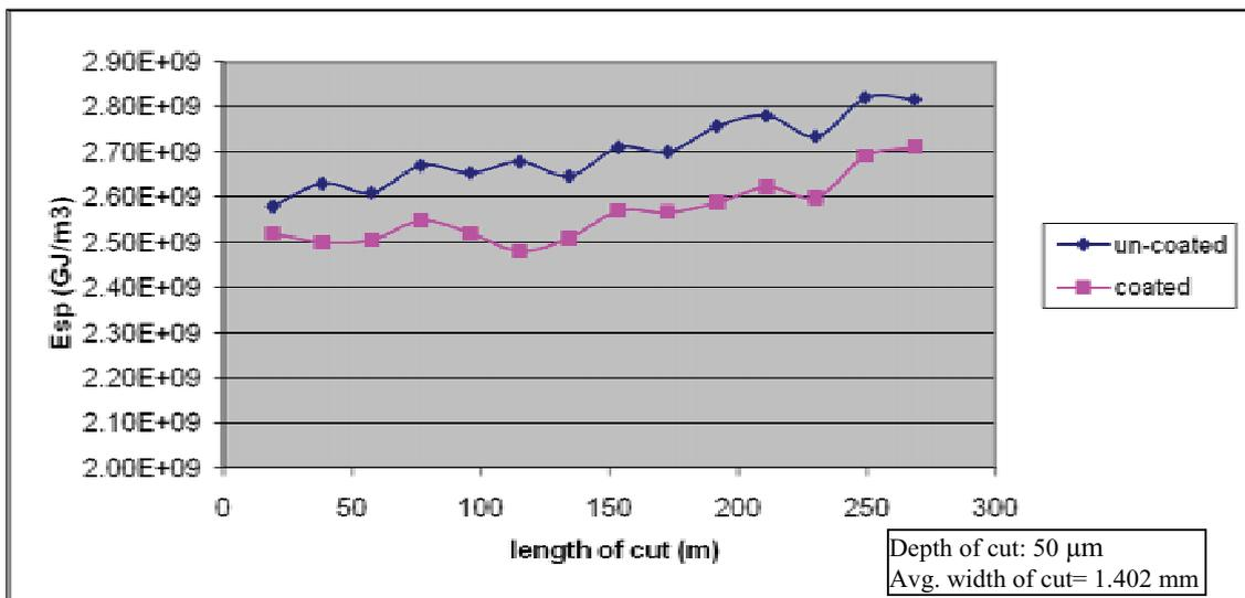
Figure 6: Variation in  $E_{sp}$  with the length of cut for the un-coated and coated teeth. Depth of cut: 50  $\mu m$ , average width of cut: 1.402 mm
