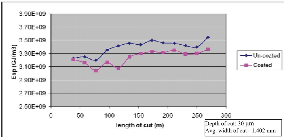
Figure 5: Variation in  $E_{sp}$  with the length of cut for the un-coated and coated teeth. Depth of cut: 30  $\mu m$ , average width of cut: 1.402 mm
