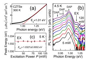
**FIG. 2.** Room temperature dependence of  $(\alpha hv)^2$  on photon energy hv (a), evolution of the PL spectrum with increasing excitation power P (b), excitation power dependence of the EX peak at 5 K (c).
