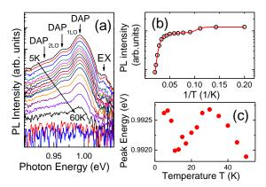
**FIG.3.** Temperature dependence of the PL spectra (a), temperature quenching of the integrated intensity of the DAP peak (o - experimental points, - fitted line) (b), dependence of the DAP peak spectral position on temperature (c).
