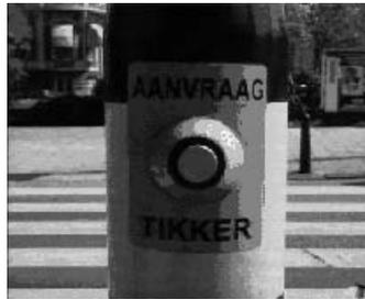
**Fig. 6.** Unclassified. In order to help the blind cross over, 'tikers' have been installed at zebra crossings, giving sonic cues to the state of the traffic lights. The sound sometimes lead to complaints from people who lived next to them, which, in turn, led to a most curious design solution: the ticking information has to be requested by pressing a button. How will the blind person find the button, or its function, the first time he or she comes here?
