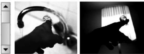
**Illustration 5:** Telebead: Moving the ring scrolls water in the tap or light in the lamp
