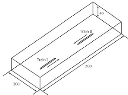
Fig.5 The aerodynamics model of two trains meeting
