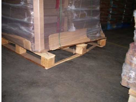
Figure 2- Broken Pallet of Pizza Boxes in Delivery Point
