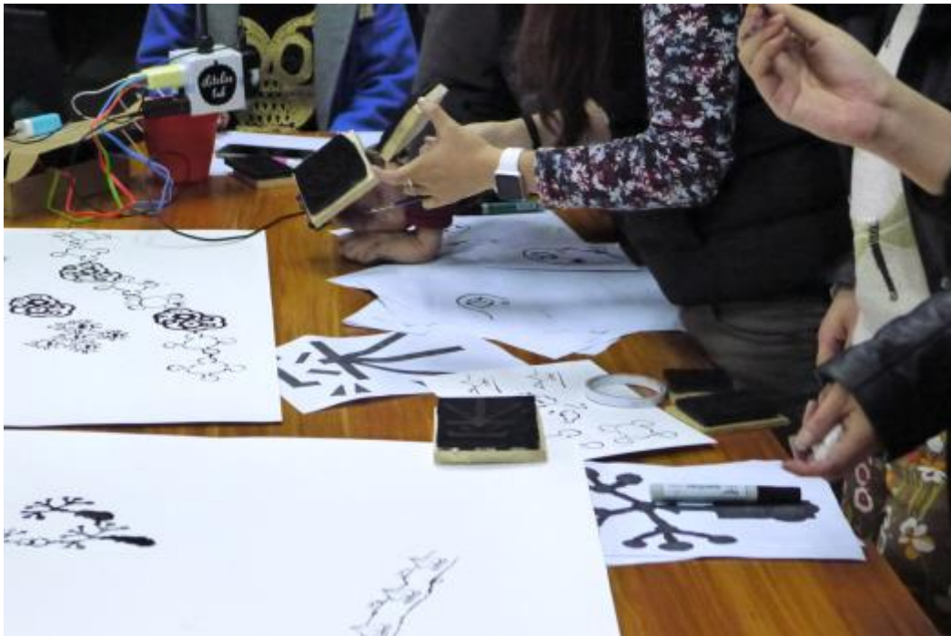
Figure 2: Laser engraved printing blocks derived from participants drawn designs.
