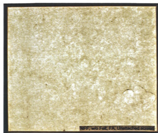
Figure 146. A sheet made with unfermented flax, without felt, with mucilage, and with a flexible laid screen.
