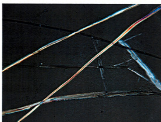
Figure 47. Fibres with rather faint cross-markings (x250).
