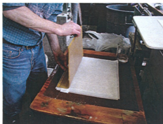
Figure 94. Couching a sheet made upon a flexible laid mould.
