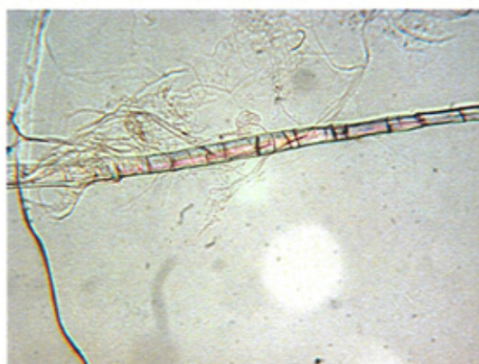
Figure 86. A fibre with clear cross- markings and longitudinal striations (x250).
