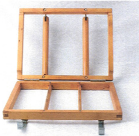
Figure 15. A supporting frame and hinged deckle having two handles.
