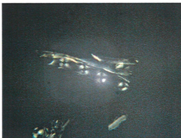
Figure 117. bordered pits under cross-polar (x250). The same sample as Figure 114.
