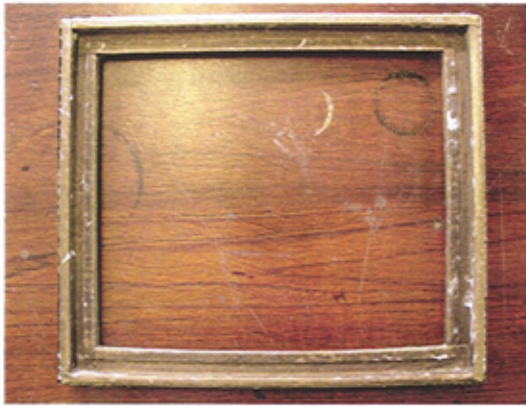
Figure 7. Deckle for the wove mould.
