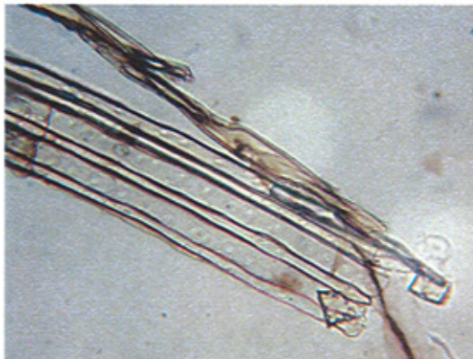
Figure 78. A bundle of longitudinal tracheids showing bordered pits (x250).
