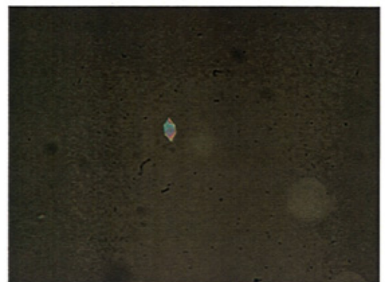
Figure 55. An elongated hexagonal shaped crystal (x400).
