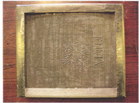
Figure 8. The deckle positioned on the wove mould.
