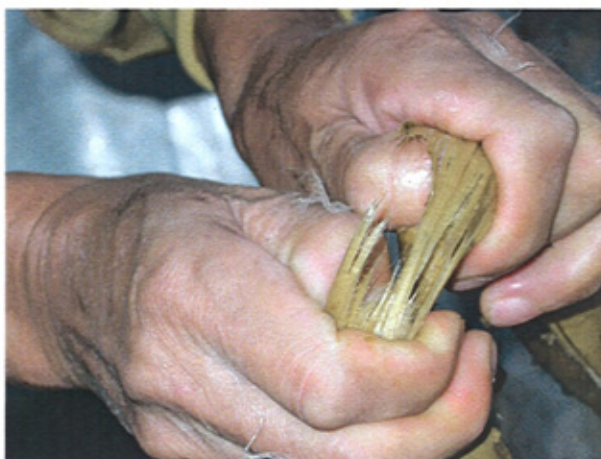
Figure 23. A papermaker checking the cooked baekpi (the picture was taken at Jangjibang, in Korea)
