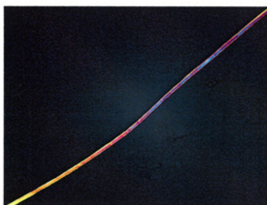
Figure 71. A fibre showing cross-markings and narrow lumen (x250).
