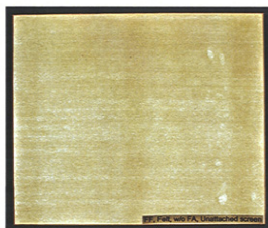
Figure 148. A sheet made with fermented flax, felt, without formation aid, and with a flexible screen.
