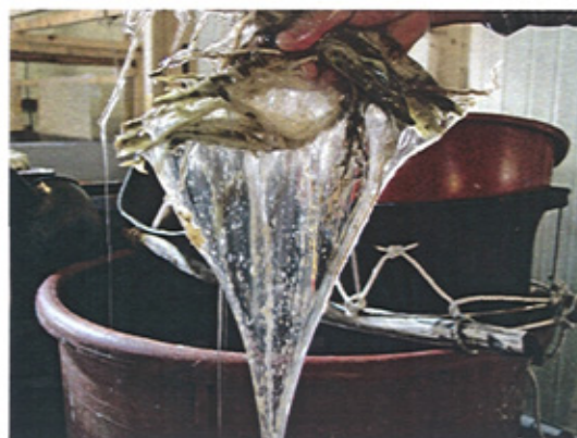
Figure 28. Clear, viscous mucilage from the crushed and soaked roots (at Jangjibang).
