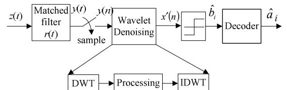
Figure 2: The DWT based receiver for the OWC system in presence of ALI.
