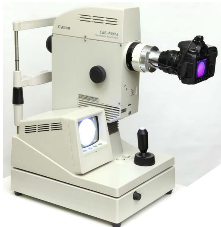
Figure 1.1. Canon CR6-45NM retinal camera with digital camera upgrade installed (Cheng et al., 2017)
