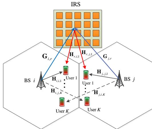
Fig. 1. An IRS-assisted multicell MIMO multiuser communication system.
