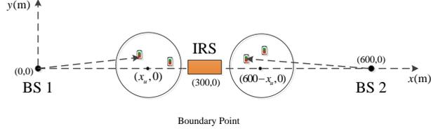
Fig. 3. The simulated two-cell IRS-aided MIMO communication scenario.
