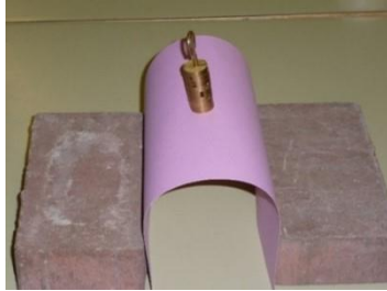
Fig. 14.2 Testing an arched structure
