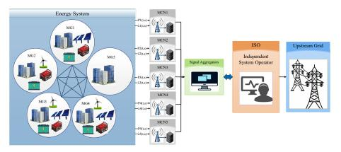
Figure 1: The schematic of the studied energy system including five microgrids fully interconnected
