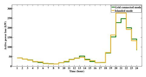
Figure 17: Total power loss with and without MGs for CS7
