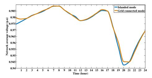
Figure 18: Total deviation of voltages obtained with and without MGs for  $\underline{CS7}$
