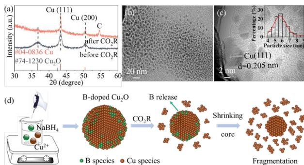
**Figure 2.** Synthesis and structural characterizations of the catalysts. (a) XRD patterns of B-doped  $Cu_2O$  catalysts before and after  $CO_2R$ . (b) TEM and (c) HRTEM images of fragmented Cu catalysts after  $CO_2R$ . The inset image in (c) is the statistic of particle size. (d) Schematic illustration of the structural evolution of fragmented Cu catalyst.
