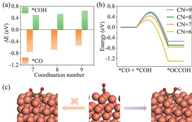
**Figure 1.** (a) The adsorption energies of  $^*CO$  and  $^*COH$  on Cu (111) surface with different CNs. (b) The reaction energies for the OC-COH coupling on the Cu (111) surface with different CNs. (c) Two competitive reaction pathways for C-C coupling. Light brown, copper; pink, hydrogen; red, oxygen; dark brown, carbon.
