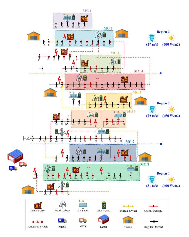
Fig. 1. Modified IEEE 118-bus distribution system structure.
