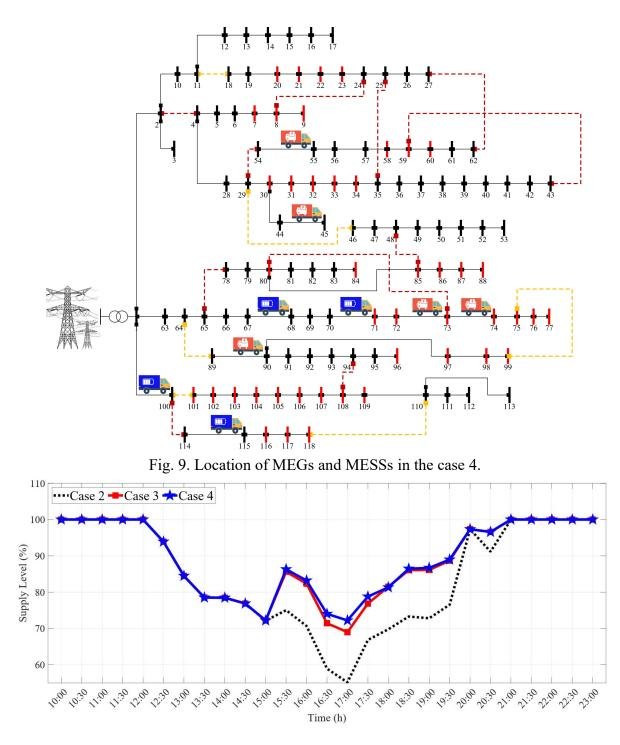
Fig. 10. Load supply curve in cases 2, 3 and 4.
