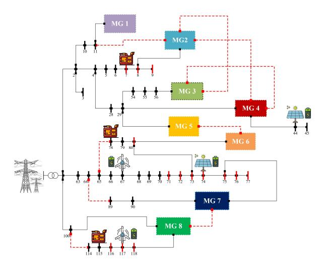
Fig. 11. Topology obtained for the network by considering proactive actions.
