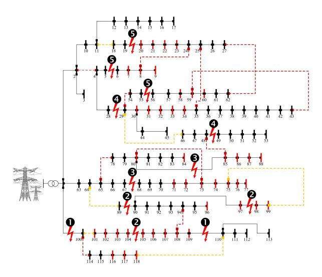
Fig. 17. Scheduling obtained for repair crews in restoration phase.
