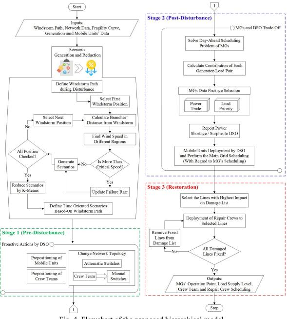
Fig. 4. Flowchart of the proposed hierarchical model.
