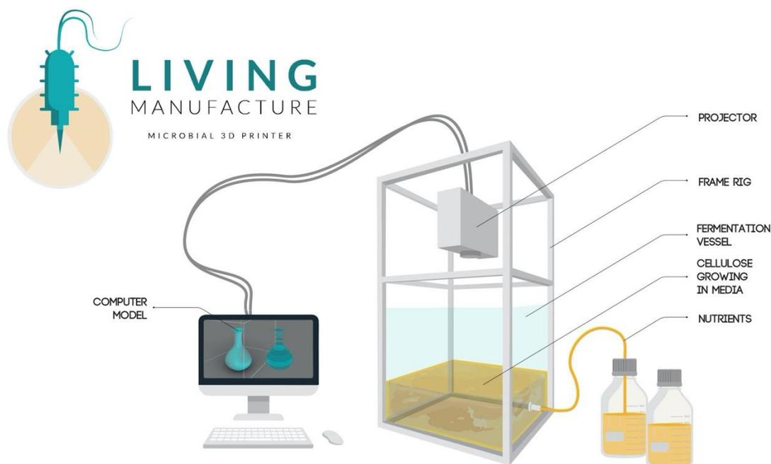
Figure 1. Concept design of bioreactor with digital and biological input.
