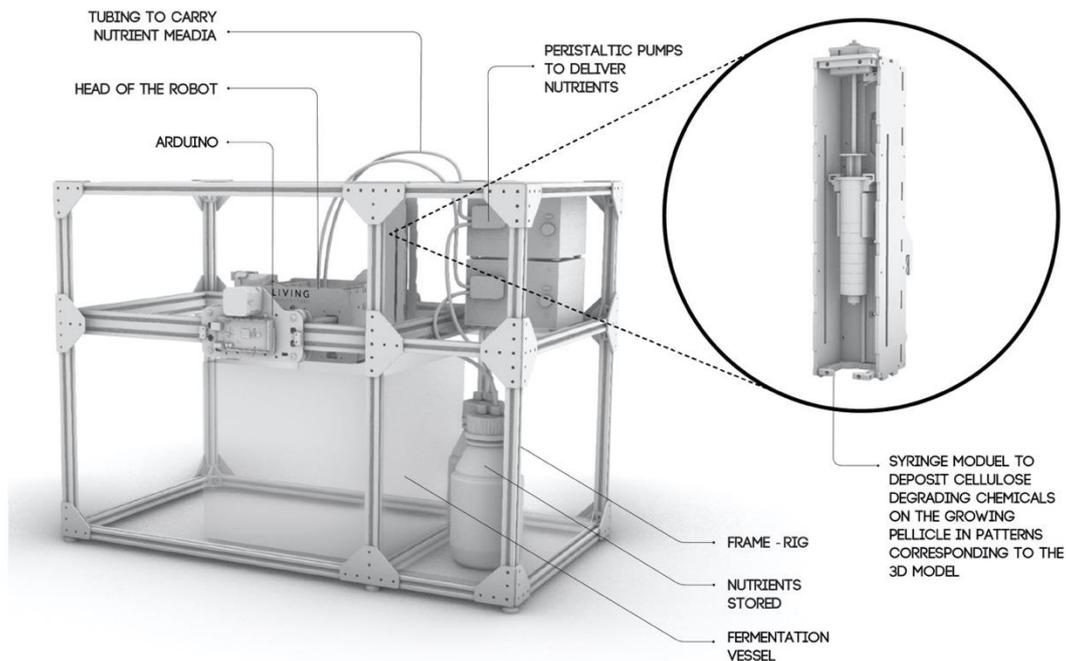
Figure 4. 3D model of the modular liquid handling robot, frame and head with the fermentation vessel below and a close-up of the syringe module.
