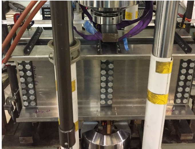
Figure 7: Shear test assembly of 40030-2WSP-8AS-2VRB.
