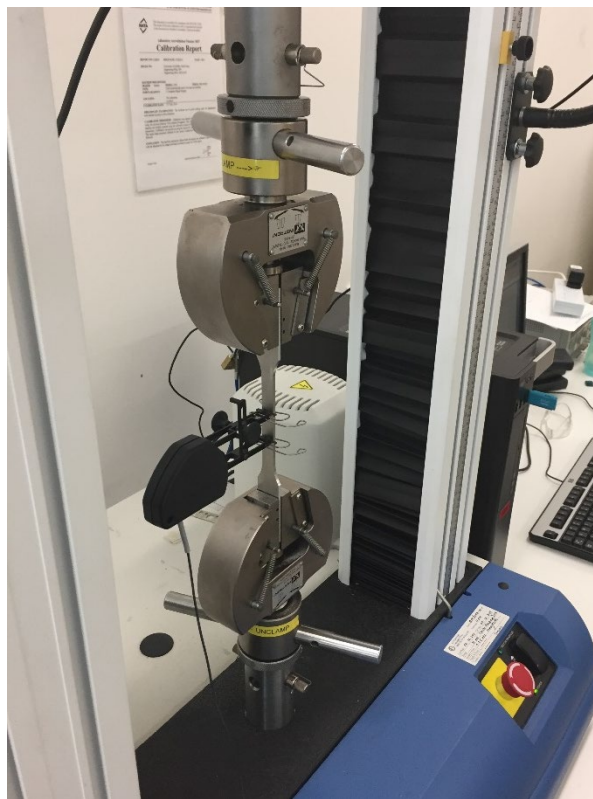
Figure 2: Tensile coupon test set-up.
