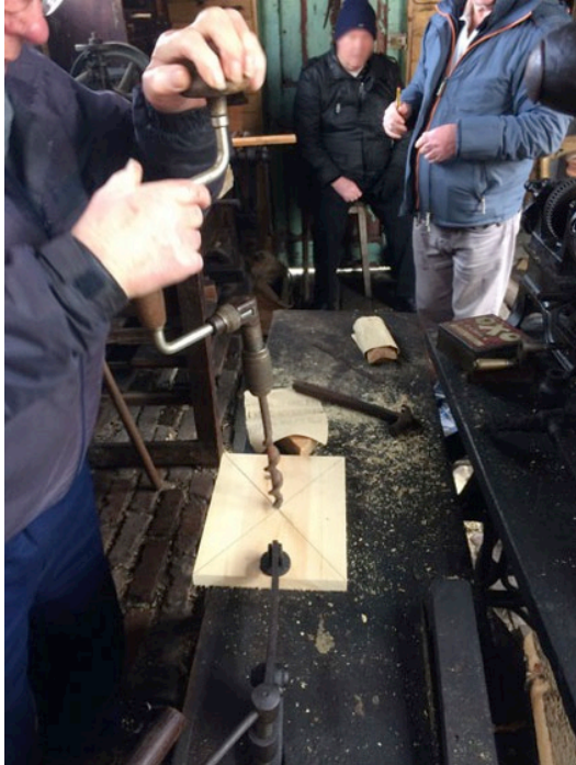
Figure 4.12: Using a hand auger in a cricket making workshop led by a participant
