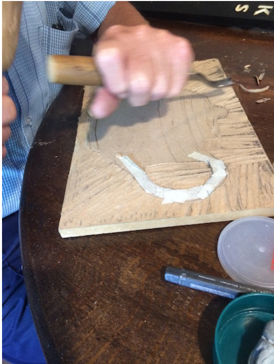
Figure 6.42: Using masking tape to protect areas of wood
