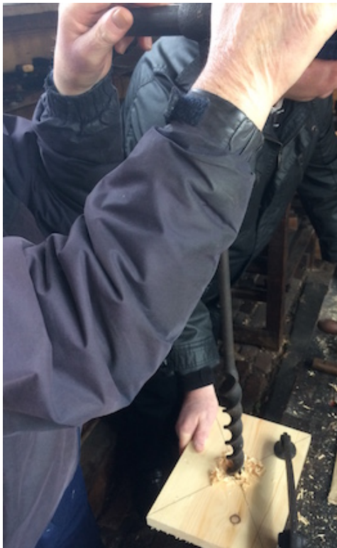
Figure 6.37: Bert making a hole in a cricket leg using a hand auger
