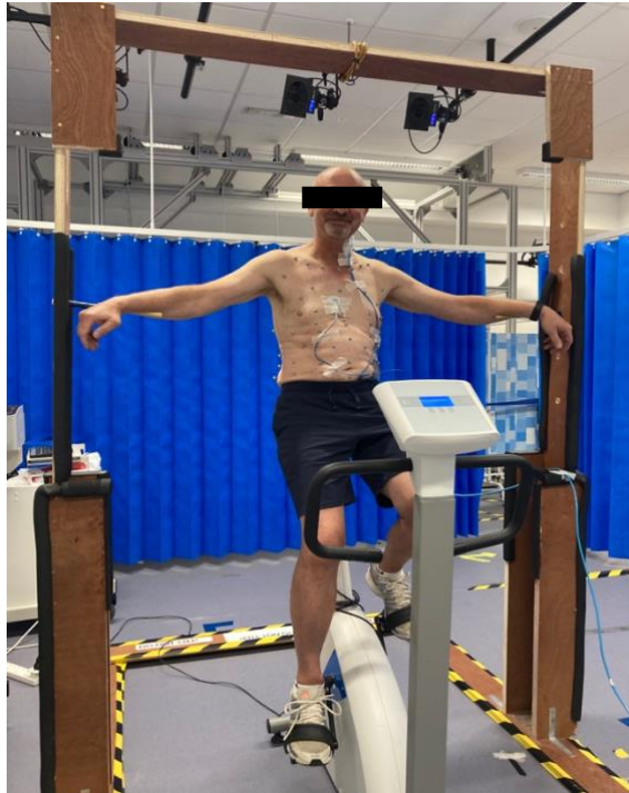
Figure 4-1. The participant set-up for optoelectronic plethysmography (OEP) measurements during inspiratory muscle loading (chapter 5) and constant work rate exercise (chapter 6). Note: PhysioFlow electrodes also attached to participant (outlined in chapter 6).
