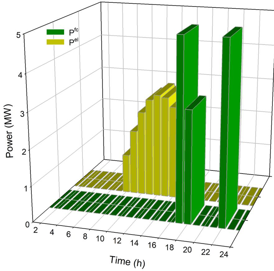
Figure 14: Performance of hydrogen storage system in CS2.
