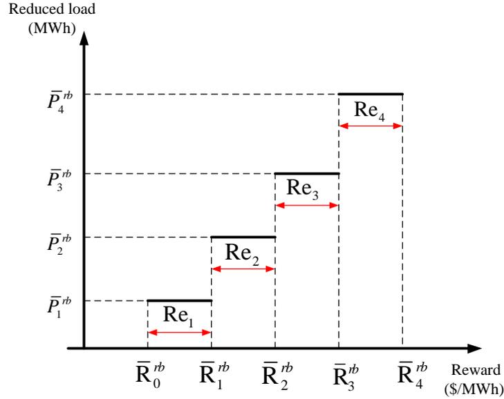
Figure 4: **Reward-based demand response operational curve.**
