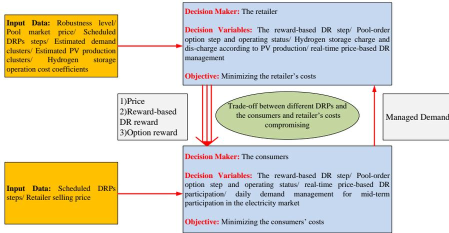
Figure 2: The flowchart of the problem optimization procedure
