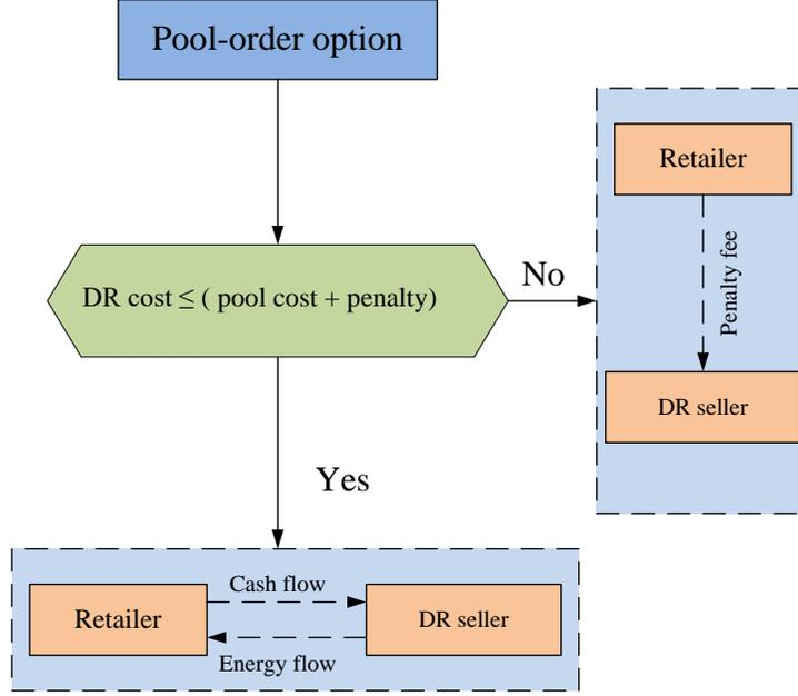
Figure 3: The schematic model of pool-order demand response
