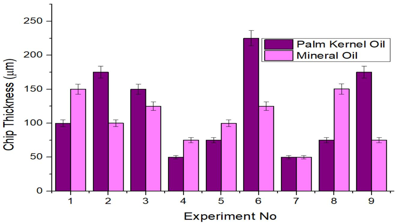
**Fig. 3:** Effect of minimum quantity lubrication on chip thickness ratio of AISI 1039 steel
