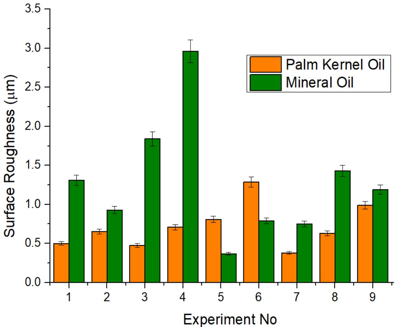
**Fig. 1:** Effect of minimum quantity lubrication on surface roughness of AISI 1039 steel
