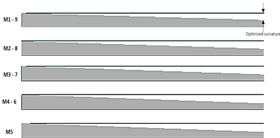
Figure. 3.18: Pictorial (symmetrical) representation of optimised mirror curvatures – M- mirrors 1- 9
