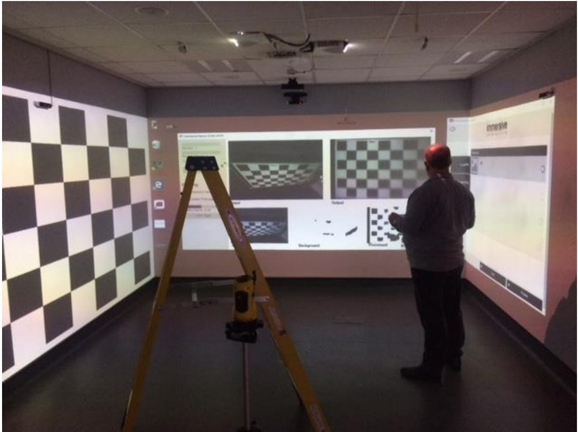
Figure 16: Technician using a grid layout of squares to ensure each wall is balanced
