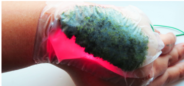
Figure 5: Prototype with embedded strips of LEDs, micro vibrator motor and Arduino. The prototype will evolve to encapsulate the vision of the concept through 3D printing or other mold making methods.
