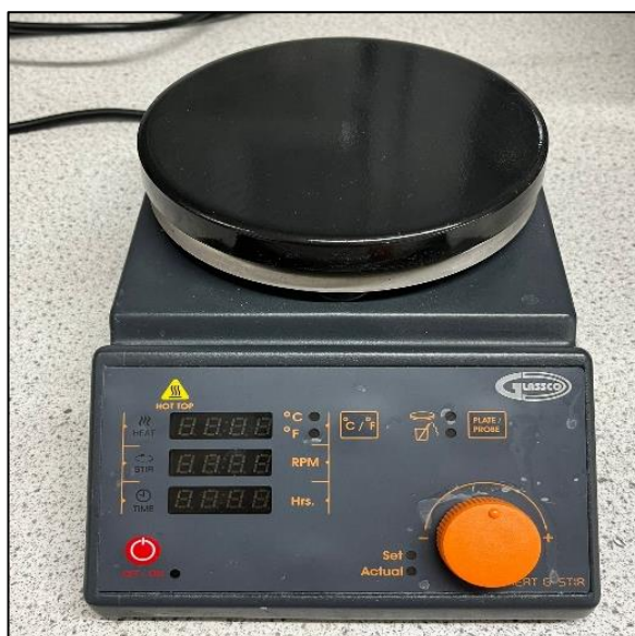
Figure 3.3: Overview of the Glassco 900.DNDG.01 magnetic stirrer with digital hotplate.
