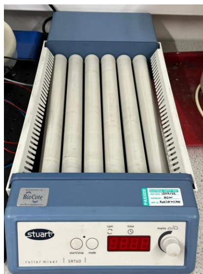
Figure 3.2: Overview of the Stuart SRT6D roller mixer equipment
