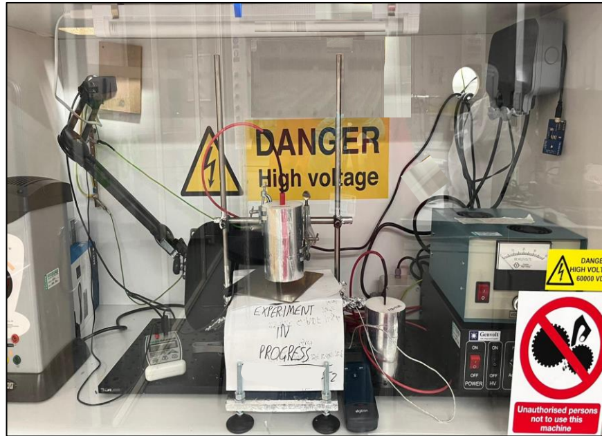
Figure 3.14: Overview of the poling experimental setup
