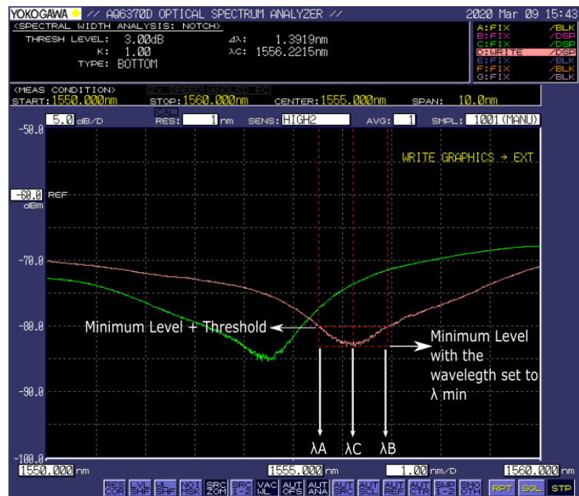
Figure 5.5 A typical spectrum as the output of the optical spectrum analyser.
