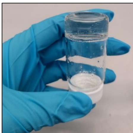
Figure 3.6 The upside-down vial containing the gel based on KELCOGEL ® F gellan gum. The gel strength and its clarity are visible.
