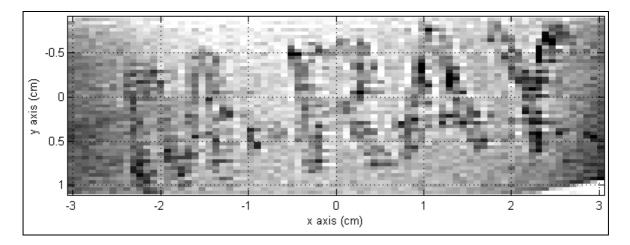
The slide was made by laser etching "M-RAY" the glass slide, and then immobilising cDNA into the etch surface before hybridising with cDNA (as described in the communication) and imaging in water. MRI details: RARE sequence, RARE factor = number of lines = 128,  $T_E = 30 \text{ ms}$ ,  $T_E^{\text{eff}} = 1726 \text{ ms}$ , 16 averages, spatial resolution = 781 x 391  $\mu$ m<sup>2</sup>, slice thickness = 1 mm, imaging time = 62 s.
