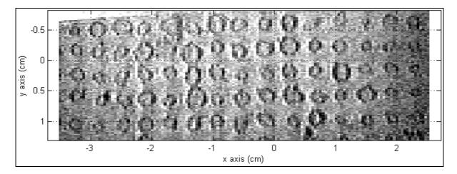
The slide was made by laser etching a 5 x 15 array and spotting with cDNA (all the same). cDNA was then spotted onto the spots directly and allowed to dry. This was subsequently washed before imaging in water. MRI details: RARE sequence, RARE factor = number of lines = 64,  $T_E = 30$  ms,  $T_E^{eff} = 975$  ms, 8 averages, spatial resolution = 1172 x 547  $\mu$ m<sup>2</sup>, slice thickness = 0.5 mm, imaging time = 15.5 s.
