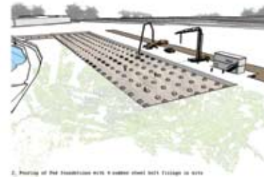
2. Pouring of the foundations with a concrete steel reinforcement
