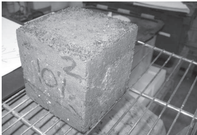
Plate 4: 10% Rubber sample at 50 freeze/thaw cycles
