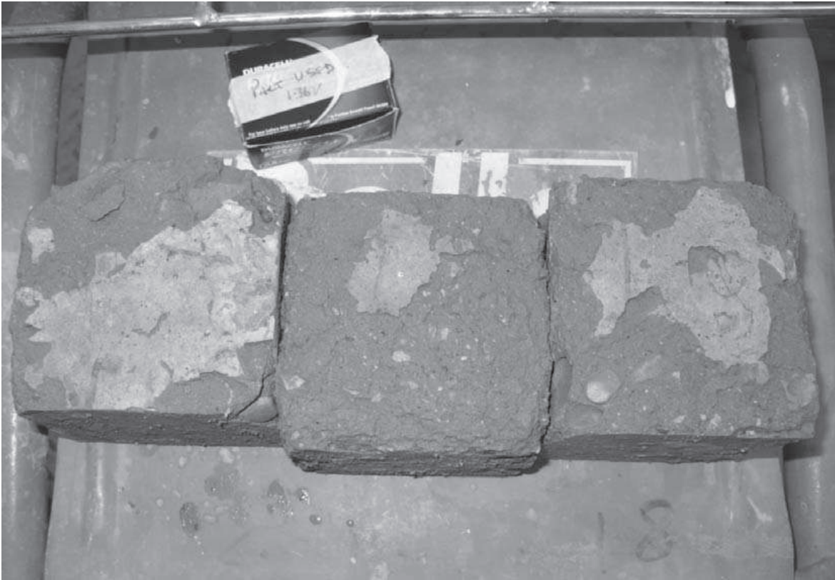
Plate 1: Plain concrete cubes at 50 freeze/thaw cycles
