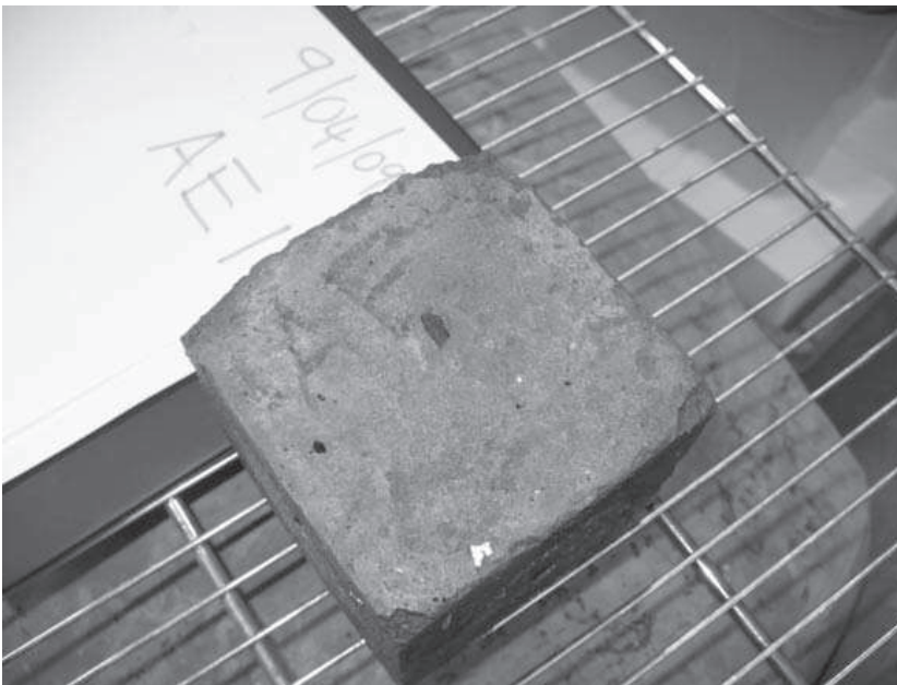
Plate 2: Air Entrained sample at 50 freeze/thaw cycles
