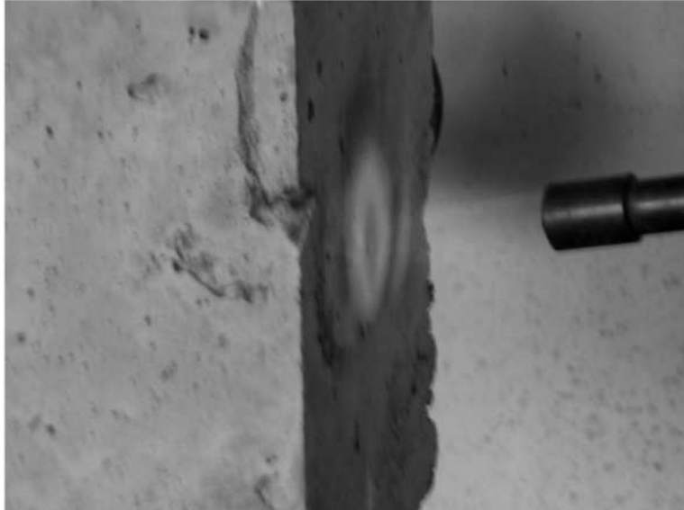
Fig3.0, 2 hour bunsen burner pilot test
