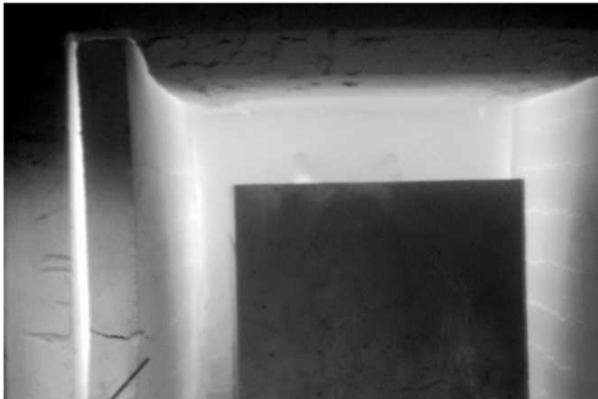
Figure 4 – Concrete cube in 1000°C furnace
