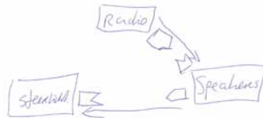
Fig. 7. A mental model drawing of the perceived network when using the Nodes design: Data is sent from the radio towards the speaker-set, which acts as a relay to an ambient light.
