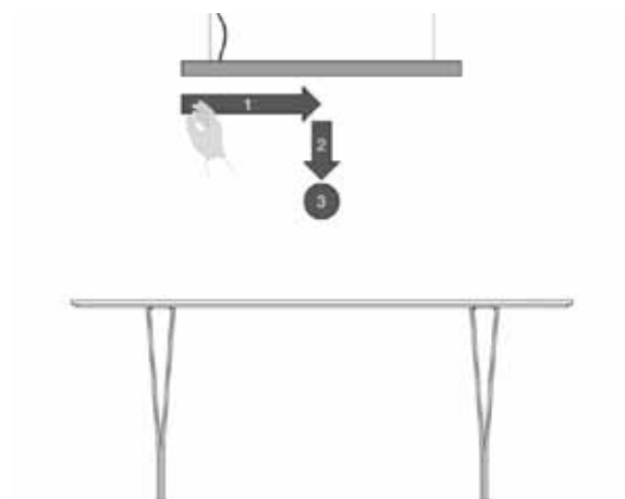
Fig. 2. Diagram showing the dining room table fixture suspended above a table. The original initiation gesture required users to: (1) move their hand horizontally from the side to just below the middle of the lamp, (2) move it vertically downwards, (3) hold it still for two seconds.
