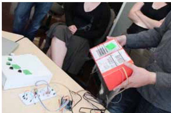
Fig. 5. Virtual ball-in-a-box haptic interface built in one day.
